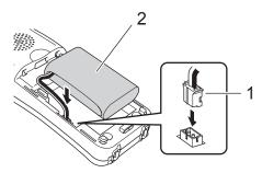
4 Place the battery in the correct position.
